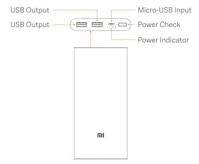
The Power Check button is not a Power button.
