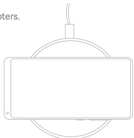
3. Keep your phone centered on the Mi Wireless Charging Pad while charging. Adjust the position of your phone if it is not charging, the green LED light should come on and your phone's status should change to "Charging" (Please refer to figure below for placement).
