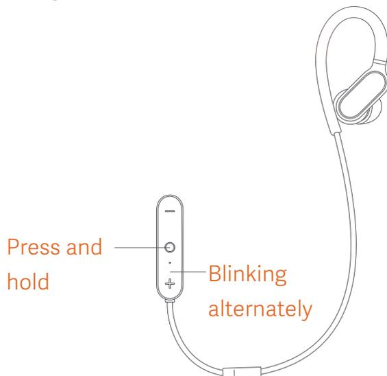
When the earphones are charging, press and hold the multifunction button until the light starts blinking alternately.
