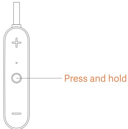
The earphones are ready to be paired when you use them for the first time. To pair again, press and hold the button until the light turns white and starts blinking.
