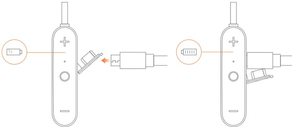
When the power is low, the light will turn red and start blinking. You'll hear a notification sound as well. Note: After fully charged, make sure the USB port is capped to prevent moisture.
